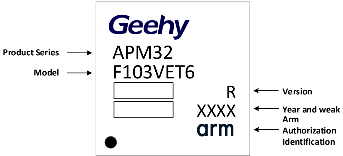
Figure 22 LQFP100 - 100 pin, 14 x 14mm package identification diagram
