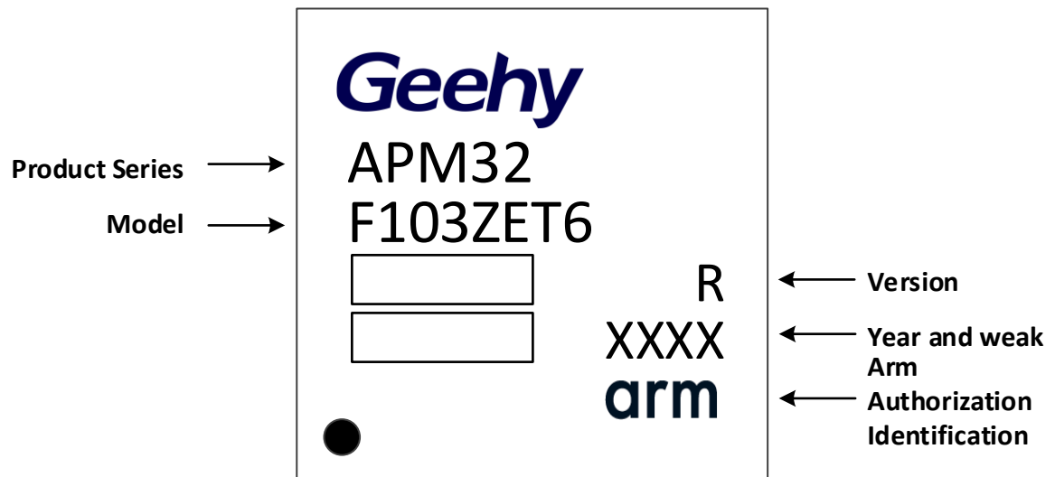
Figure 19 LQFP144-144 pin, 20 x20 mm package identification diagram
