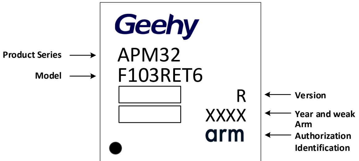
Figure 25 LQFP64 - 64 pin, 10 x 10mm identification diagram
